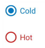
Two RadioButton views inside a RadioGroup . RadioGroup allows us to control a group of radio buttons, and make sure only one is checked
